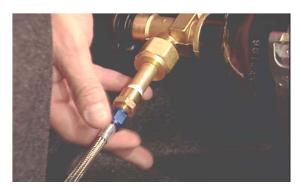
Route the 14' supply line toward the front of the vehicle. Make sure the area is clear from any moving suspension parts or exhaust piping. Use clamps, zip ties, or other hardware to secure this line. Finish securing the supply line allowing it to enter the engine compartment from under the vehicle.
