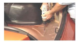
Replace the trunk interior. Punch holes through the carpet for the mounting bracket bolts.
