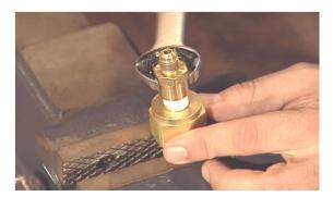
Place the Teflon Washer inside the large threads of the CGA-320 adapter. Then tighten securely to the CryO2 tank using a 11/16" wrench or an adjustable crescent wrench.
