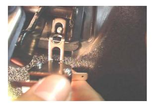
Using two wire connectors, prepare two wires for the micoswitch to activation switch circuit. Place the connectors over the terminals on the microswitch and route accordingly.
