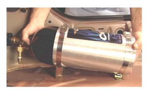
Remove the tank from the location. Using a 5/16" drill bit, drill holes through each mark.
